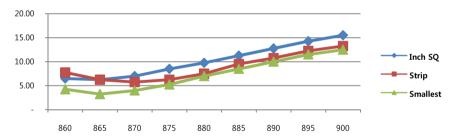
•INCH SQ reads up to 1.5 meters on metal, 40% shorter than SMALLEST, but same as STRIP. Though not best performing among similar size tags, its performance is most stable and consistent, as its slow and gentle slope of sensitivity curve shows.
