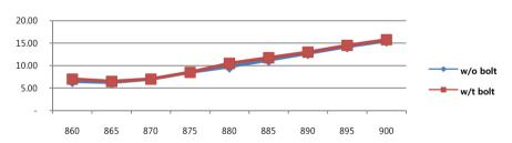
•INCH SQ reads SAME, regardless of whether fastened with metal bolt in a hole (located at center of tags) or not, because it was originally designed as assuming metal bolt in. Stainless steel M4 bolt with round head is best fit for INCH SQ with NH (Normal hole) and DH (Dish hole) both.
